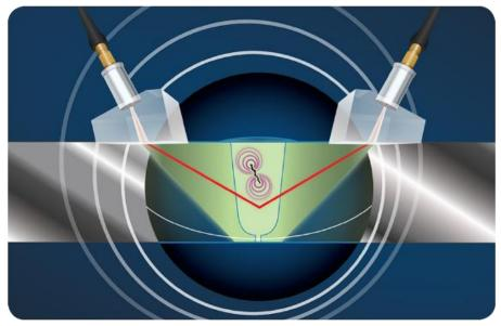
Time of Flight Diffraction (ToFD)
